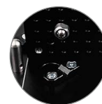
Pallet in repeatable three-point set-up
